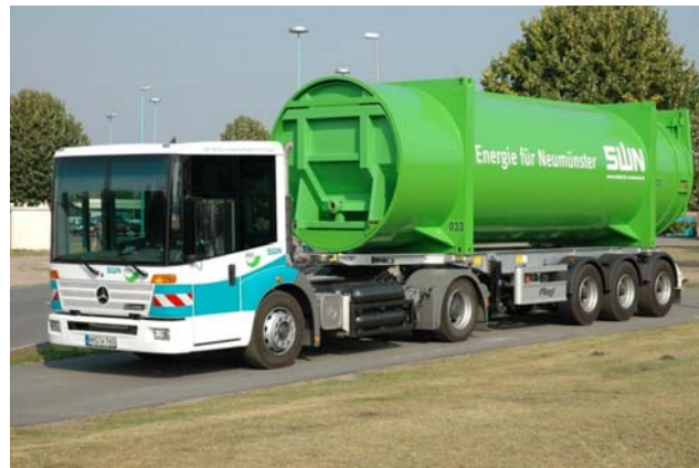
The photo below shows an MB Econic tractor fueled by methane and being used in Germany to haul waste.
