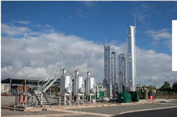
Biomethane to Grid – we can upgrade and inject the fuel into the National Gas Grid where it can be used in higher efficiency energy generators.
