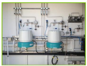
Elster Gas Chromatographs for Biomethane CV, Ofgem C6+ analysis and GS(M)R compliance
