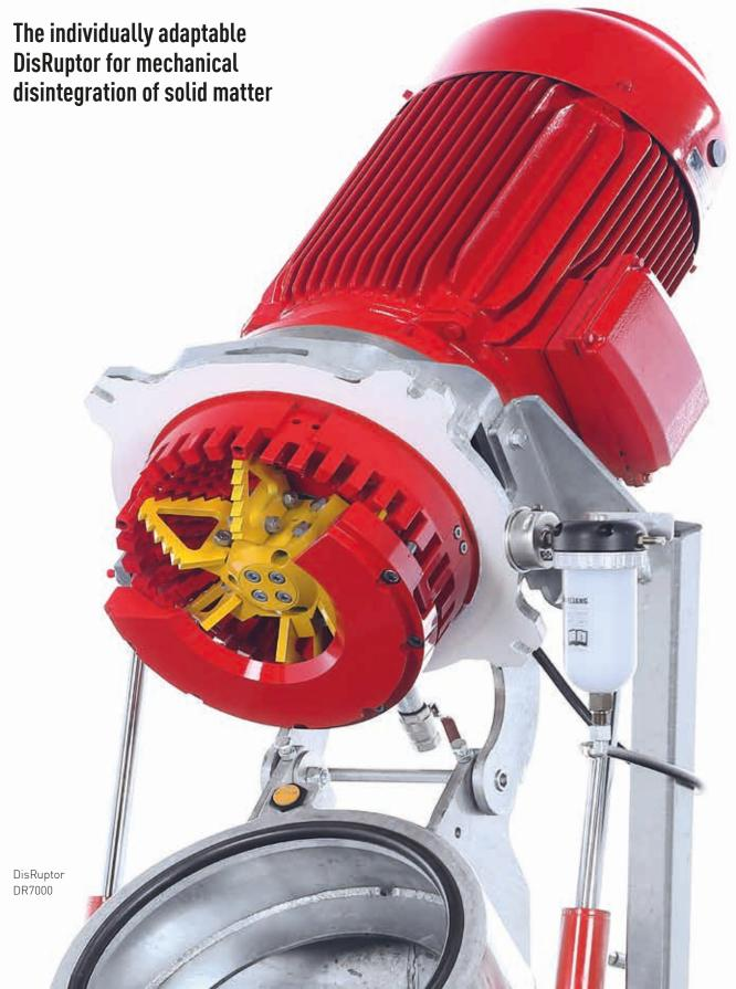
Optimal substrate disintegration is key for determining biogas yield. This is why Vogelsang also offers a mechanical alternative for disintegrating substrates: the flexibly designed DisRuptor. The reduction of the particle size and the simultaneous defibering increases the surface area of the solid matter used. This helps bacteria reach the nutrients better, accelerates conversion and increases the gas yield.
