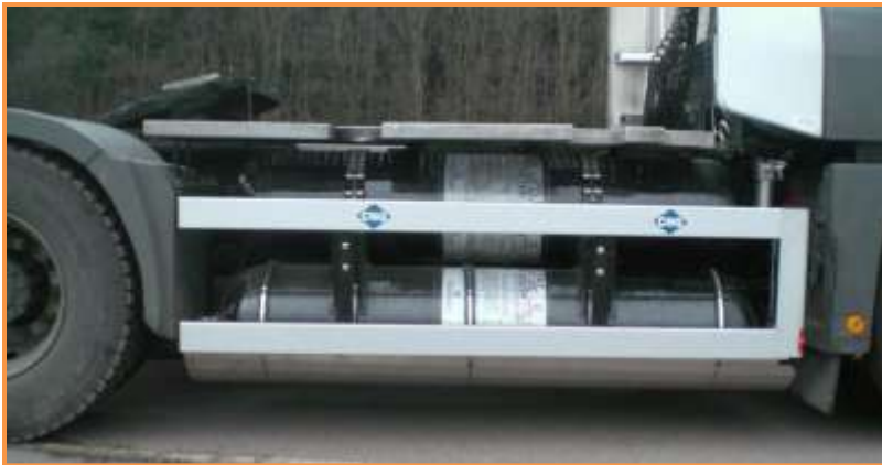
250 bar CNG storage
