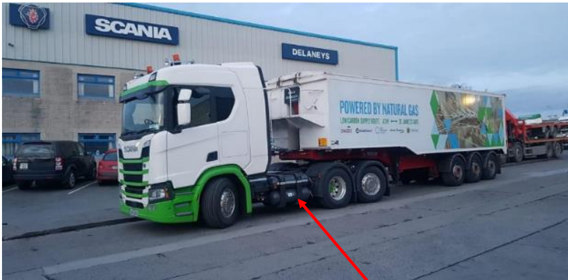
CNG Storage cylinders between the front 2 axles
